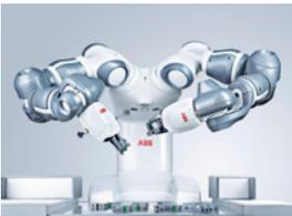
**Collaborative robots<sup>24</sup>** or “cobots” are robots designed to work alongside and in partnership with humans.
