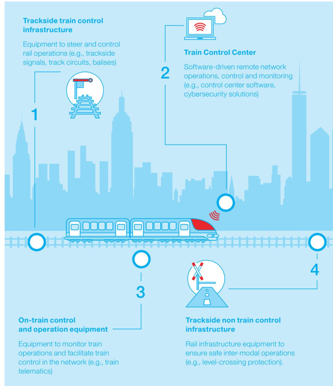
The train control and signaling segment provides all elements to safely operate and monitor a rail network and to utilize the infrastructure capacity efficiently. The signaling product space is highly complex and includes various physical assets along the tracks, within trains, and in remote control centers – all of which need to be inter-connected. While today, the high variety of an OEM's product
