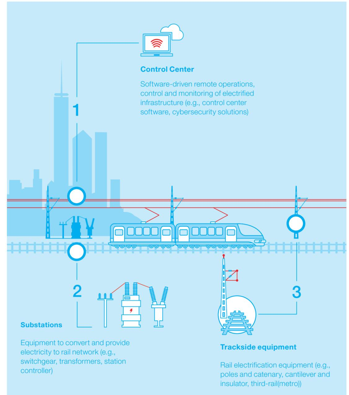
The rail electrification segment is comprised of all elements to convert and deliver electric energy directly to trains. Substations convert energy from national networks into the right frequency and voltage used in rail operations. For energy transmission along the track, two main systems dominate – catenary in mainline operations and third-rail in metro systems. Control centers
