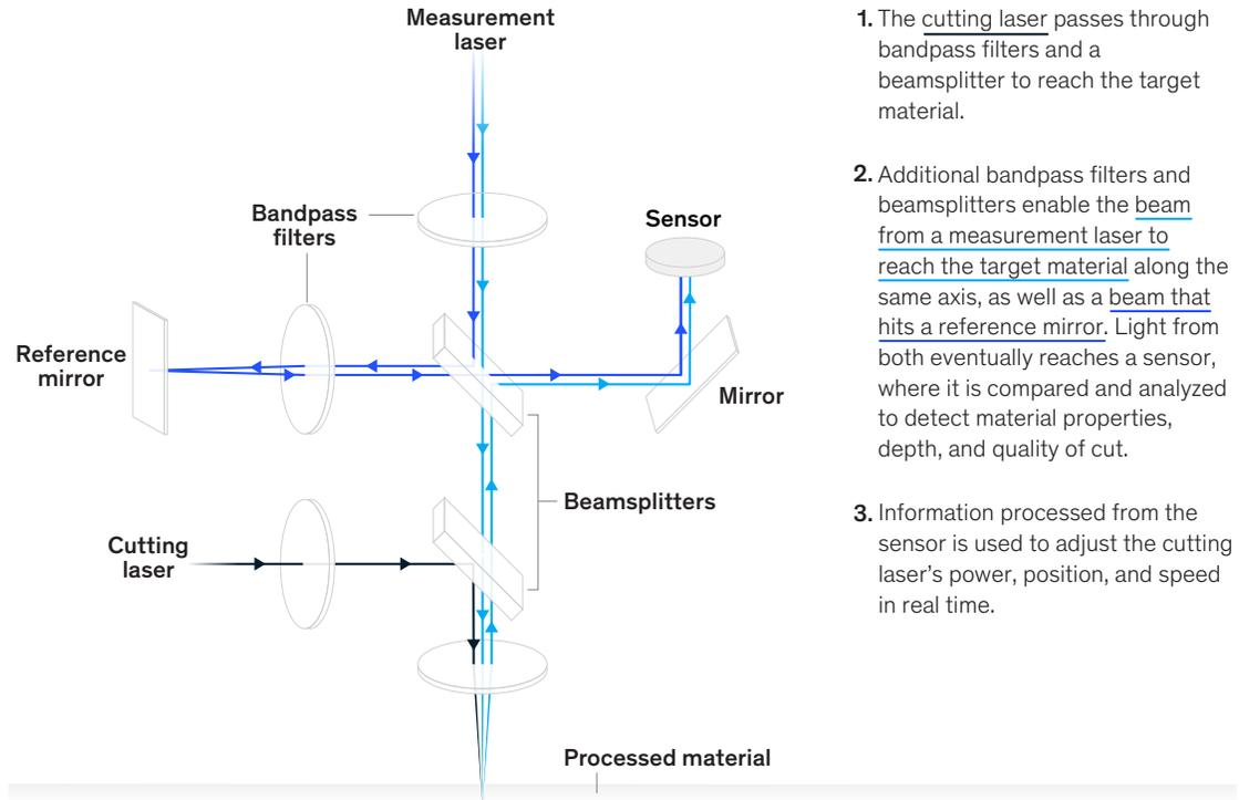
1. The cutting laser passes through bandpass filters and a beamsplitter to reach the target material.
