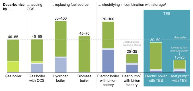
1. Ranges reflect representative fuel prices. Gas (USD 6–12/mmBTU), electricity (USD 25–50/MWh), biomass (USD 200–350/t). In the hydrogen boiler case, hydrogen production costs amount to USD 2.1–3.2/kg of hydrogen.
