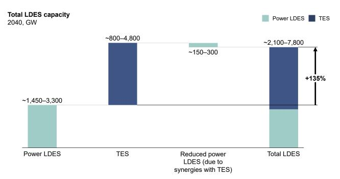
introduction of TES can help improve system efficiency and reduces power LDES needs by around 10 percent. The introduction of TES increases the potential of LDES technologies to a total between 2 and 8 TW and the overall market size to USD 1.7 trillion to USD 3.6 trillion by 2040.
