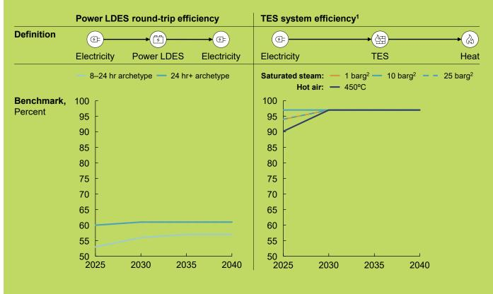
1. System efficiency is defined as the product of charging and discharging efficiency. 2. Gauge pressure (pressure in bars above ambient or atmospheric pressure).
