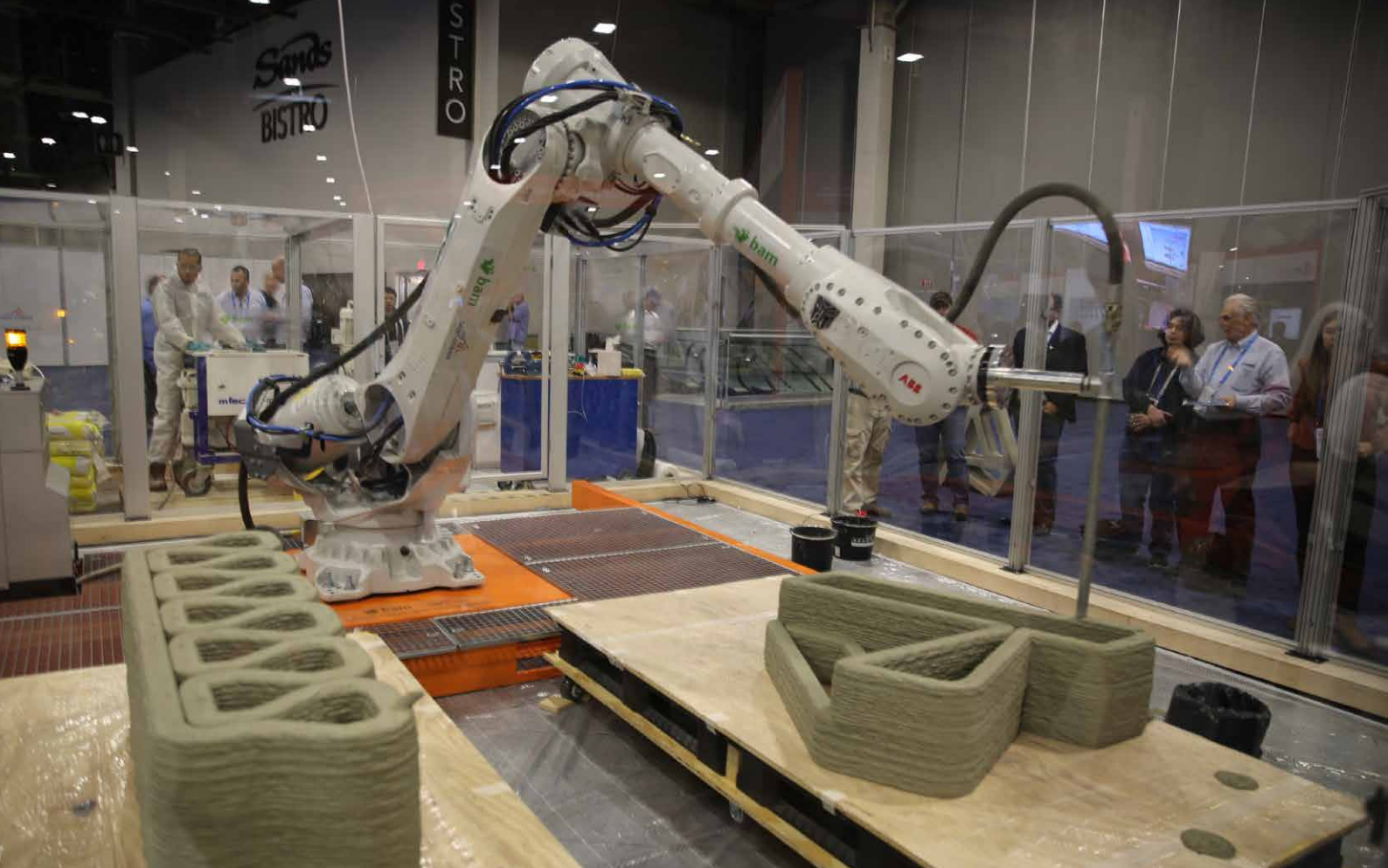
Courtesy of Autodesk: Royal BAM Group's BAM Infra and Saint-Gobain Weber Beamix demonstrate the use of a 3-D printing robot for offsite manufacturing for construction.
