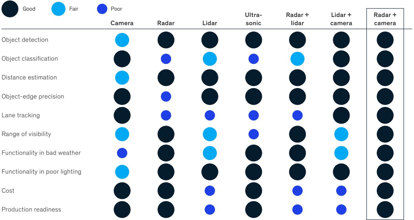
**Radar and camera most likely combination in next 5–8 years, although solid-state lidar and camera<sup>1</sup> will be dominant in the long term when proved and integrated into mass-production designs**
